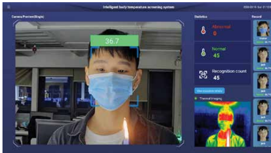
System Captures and traces forehead only, ambient temperature abnormal target (lighter, cigarette,etc) do NOT influence the accuracy
